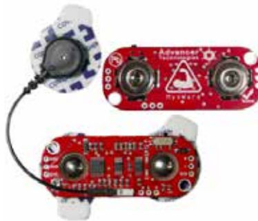
Figura 1. Sensor MyoWare AT-04-001 de Advancer Technologies
